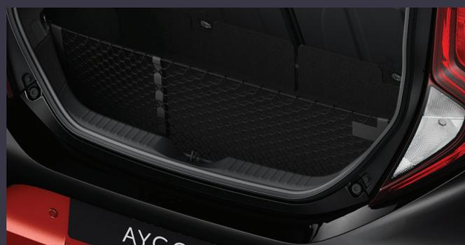
Strong, woven, black nylon net with two compartments for holding small items securely in your car's boot area. The net fixes neatly on to pre-fitted side and floor hooks.
